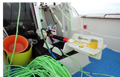
Geometrix G882 magnetometer used in the surveys
