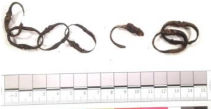
Figure 9. Image shows wrought iron chain link
